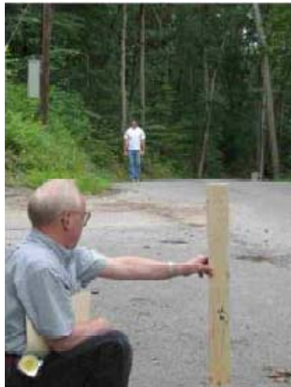
Sight distance measurement at intersection of Bayberry Rd and Heald St
